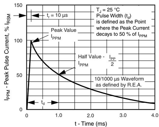
Figure 3. Pulse Waveform
