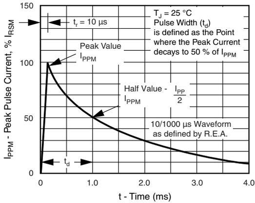
Figure 3. Pulse Waveform
