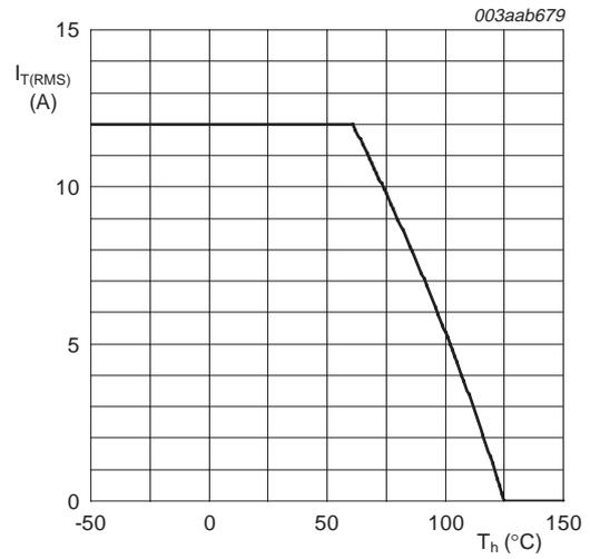
**Fig 5. RMS on-state current as a function of heatsink temperature; maximum values**
