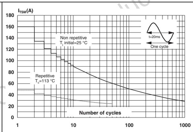
**Figure 7. Non repetitive surge peak on-state current (sinusoidal pulse width  $t_p < 10 ms$ ) and corresponding value of  $I^2t$**
