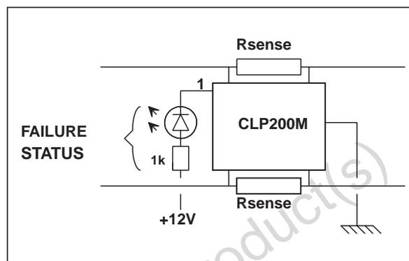
If a surge exceeding the maximum ratings of the CLP200M occurs on the line, the device will fail in a short-circuit state.
