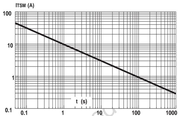
**Fig. 40 :** Maximum peak pulse current versus surge duration
