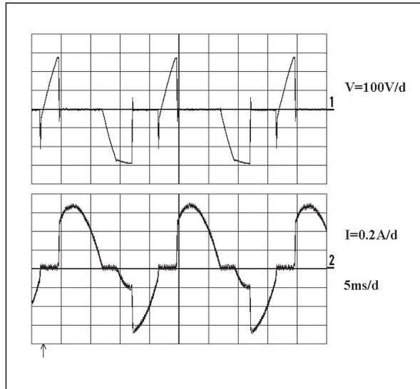
**Fig. 18 :** CLP200M response to the induction test (Test 3b).
