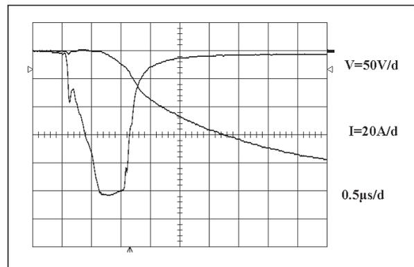
Figures 14 and 15 show that the remaining overvoltage does not exceed +/- 260 V. The CLP200M switches on within 0.7 µs and withstands the 100 A given by the CCITT K20 generator.
