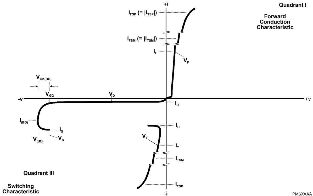
**Figure 1. VOLTAGE-CURRENT CHARACTERISTIC**
