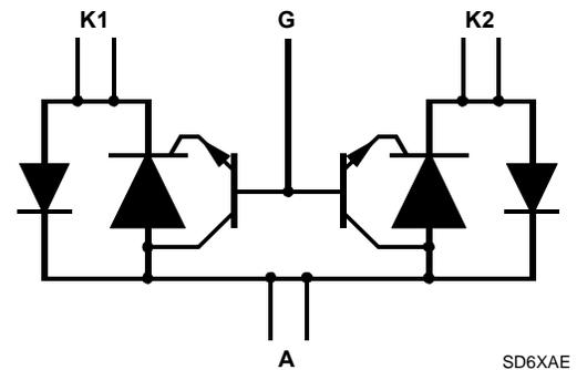
Terminals K1, K2 and A correspond to the alternative line designators of T, R and G or A, B and C. The negative protection voltage is controlled by the voltage,  $V_{GG}$ , applied to the G terminal.
