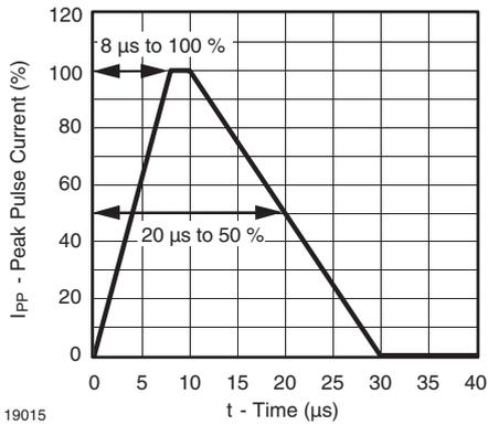
Figure 1. Pulse Waveform 8/20  $\mu\text{s}$  acc. IEC 61000 - 4 - 5
