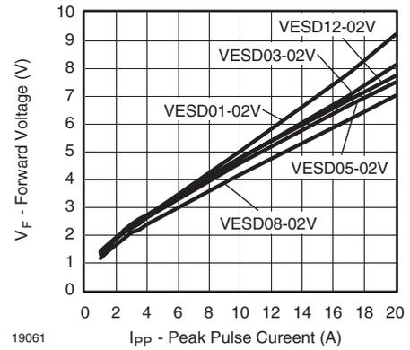
Figure 6. Typical Forward Voltage vs. Peak Pulse Current
