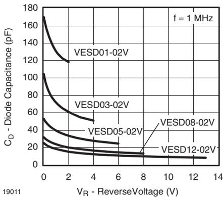
Figure 2. Typ. Diode Capacitance vs. Reverse Voltage
