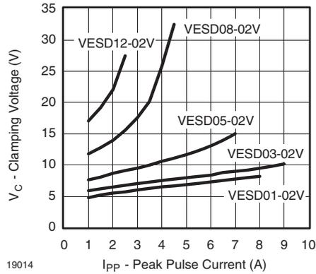
Figure 3. Clamping Voltage vs. Peak Pulse Current
