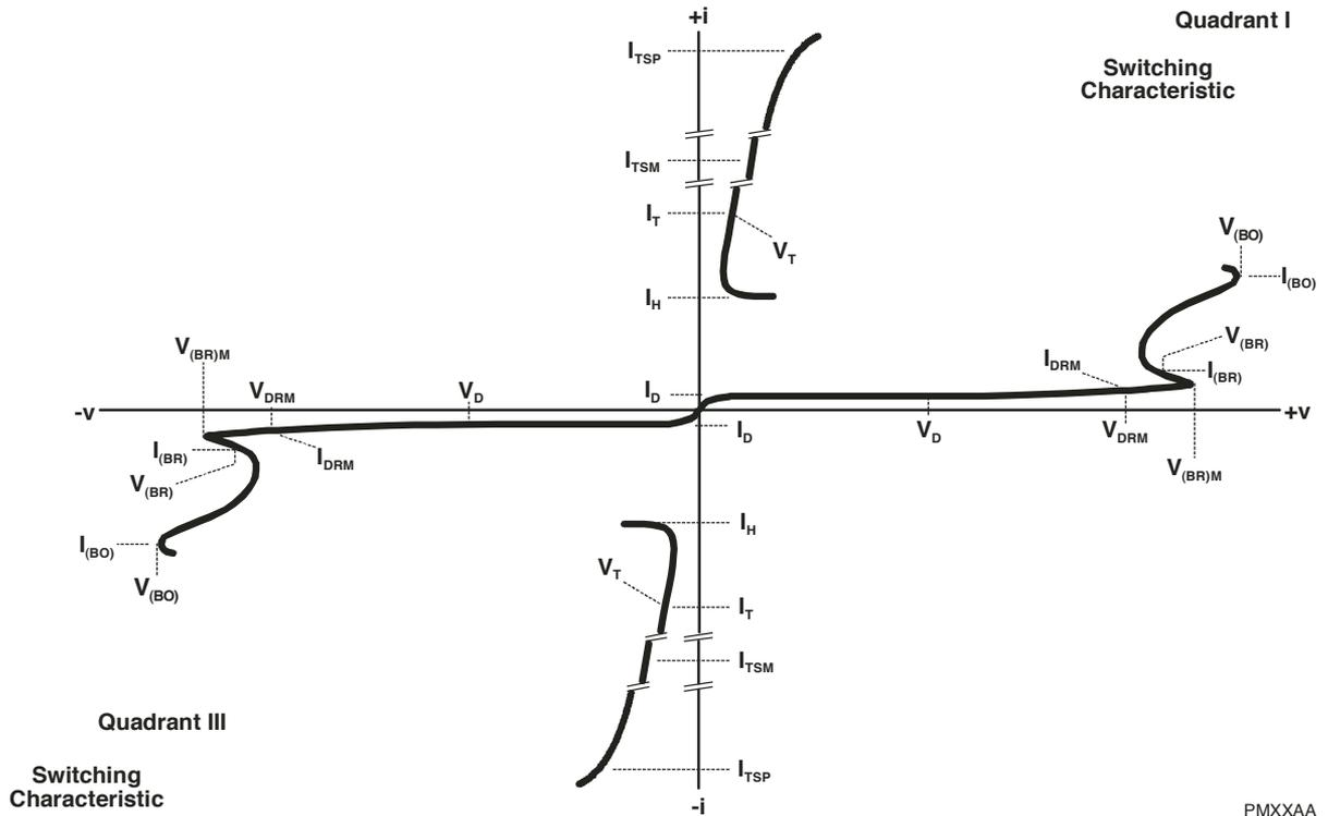
Figure 1. Voltage-Current Characteristics for any Terminal Pair
