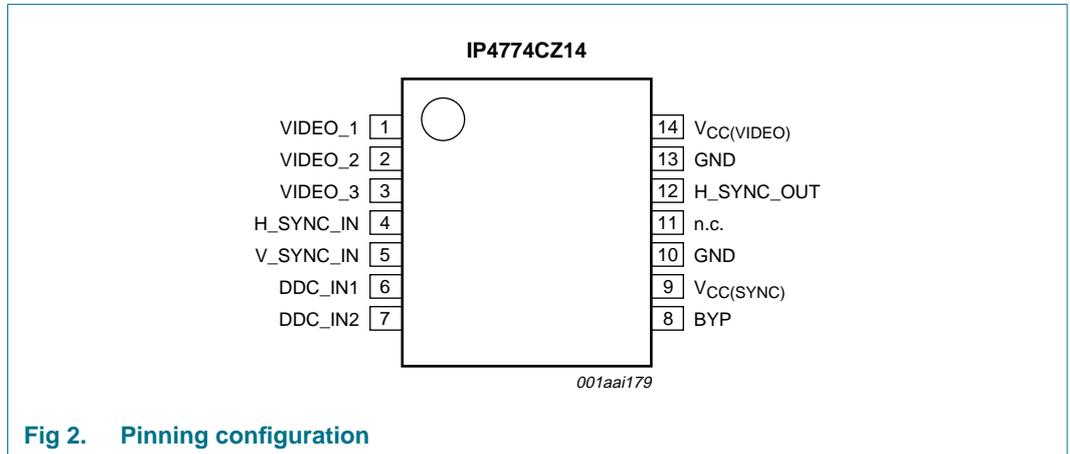
Fig 2. Pinning configuration
