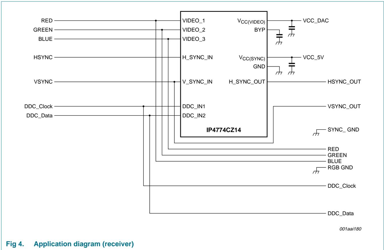
Fig 4. Application diagram (receiver)
