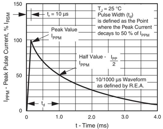
Figure 3. Pulse Waveform
