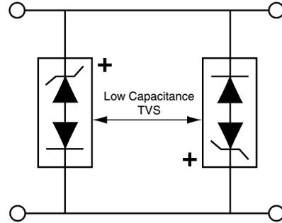
**Application Note:** Device must be used with two units in parallel, opposite in polarity as shown in circuit for AC signal line protection.
