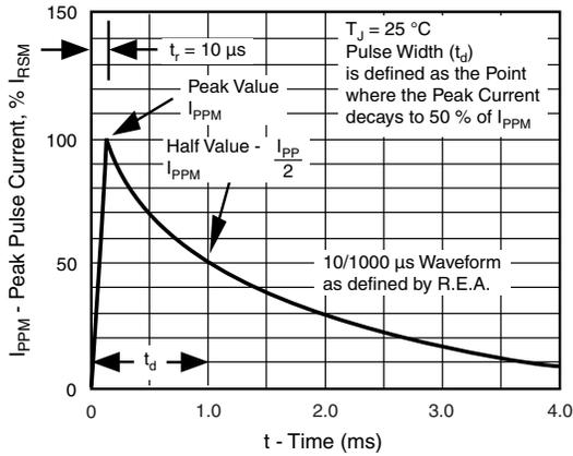
Figure 3. Pulse Waveform
