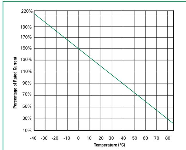
The average time current curves and Temperature Derating curve performance is affected by a number of variables, and these curves provided as guidance only. Customer must verify the performance in their application.
