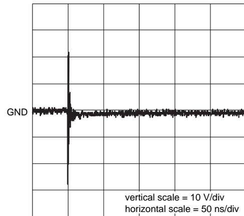
clamped -1 kV ESD voltage waveform
