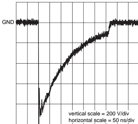
unclamped -1 kV ESD voltage waveform
