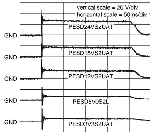
clamped +1 kV ESD voltage waveform
