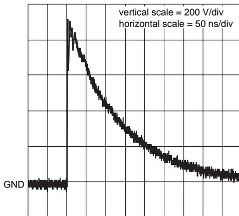
unclamped +1 kV ESD voltage waveform
